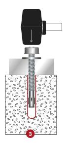
Using a hammer, tap the anchor into the hole until the washer contacts the item being fixed into the concrete.
