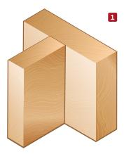
Align the supported beam with the supporting beam, ensuing both are vertically straight and all edges match up.
