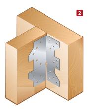
Place a pair of Multigrips at right angles on each side of the supported beam. Secure each Multigrip to its respective timber member using either Milsons 3.15 x 30 mm Nails or HWF 12G x 35 mm Screws.
