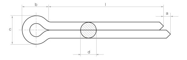
The Cotter Pin has two main measurements, the diameter, and the effective length. The easiest way to obtain these measurements is by using a pair of Vernier Calipers.
